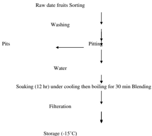
**Fig (2):** Extraction of date juice flow diagram (Shubbar, 1981).
