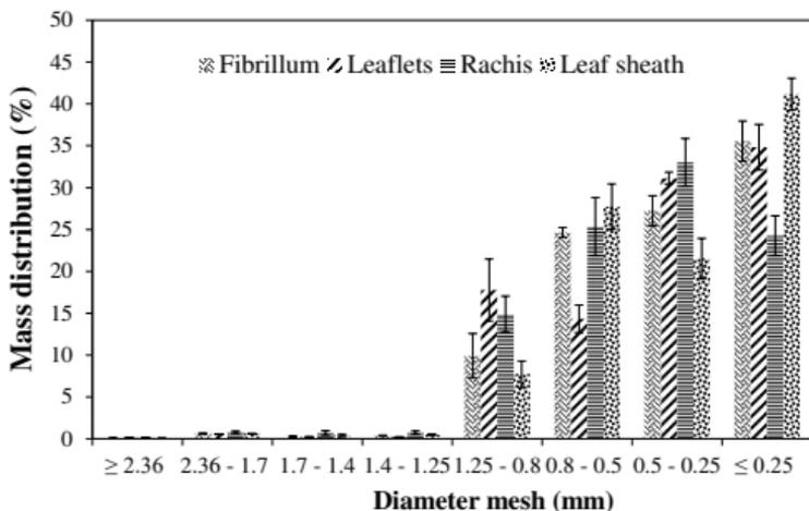
Fig. 2. Granulometric repartition of date palm by-products hammer milled through a 3 mm diameter me
